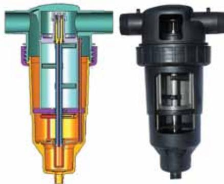
dynamic nozzle drive that does not require electric motors, limit switches, gearboxes, hydraulic pistons or any external shaft seals to operate. Available with inlet sizes in 2” or 3” (NPT/ BSP) and a flow range of 20 to 220 gpm (1.3 to 13.9 l/s), the V-200PA operates within a pressure range of 30 to 150 psi (206 to 1034 kPa). With an especially compact footprint for small areas, the V-200PA offers a wide range of filter screens from 1500 to 10 micron.
