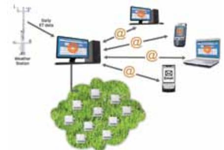
Citygal is a web based, stand alone irrigation management system that lends itself to be managed from any computer without the need to install any specific software, avoiding the necessity to set up any form of power supply, as the device operates solely on battery power.
