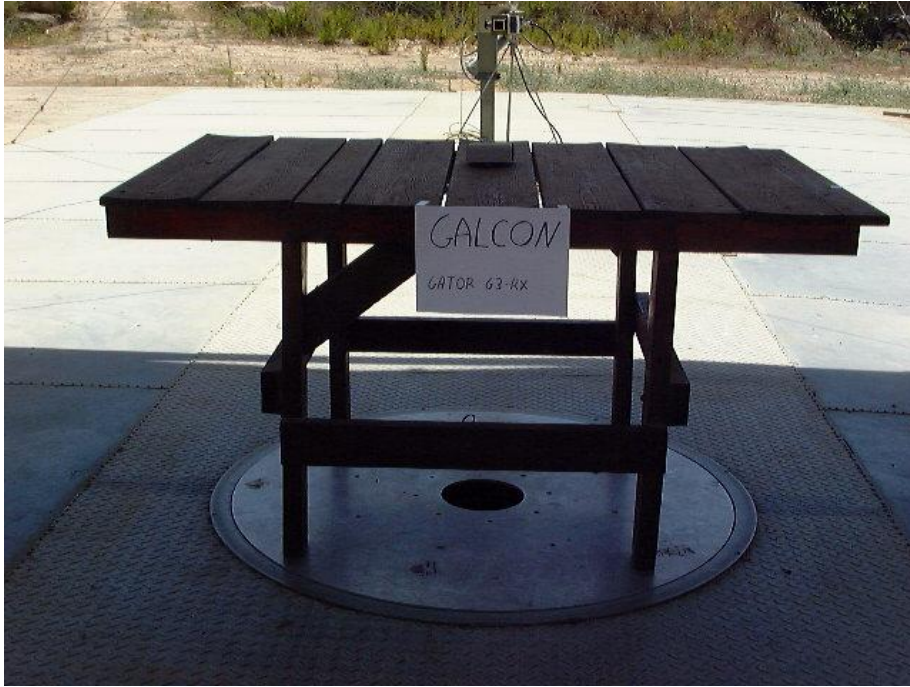
Figure 4. Radiated Emission Test
